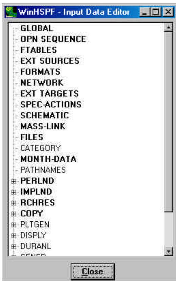
Double-clicking on a block or table name produces another window containing a grid for editing the parameters of that block or table.
